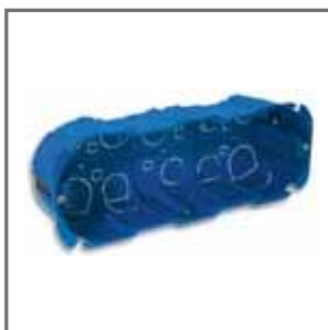
256CG Scatola rettangolare per pareti cave interasse viti 158,5mm Rectangular box for hollow walls screws fixing centres 1058,5 mm 7 mod
