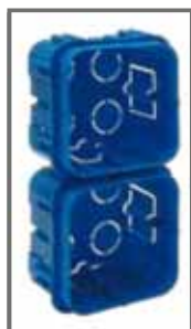
2502+2502 Scatole quadrate per pareti in muratura interasse viti 60mm - accoppiabili Square boxes for brickwork walls screws fixing centres 60 mm - they can be ganged 1-2 mod
